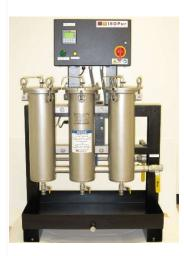
The equipment comprised the ISOPur BCA<sup>™</sup> purification system with associated controls and monitoring mechanisms. The PLC control option facilitated efficient and automated
