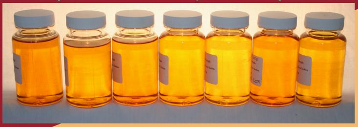
Total Run Hours 31,472 In Service Time 7.8 years ISO Codes 15/13/09 RPVOT 82% Varnish Potential 10 Gravimetric Patch - 39 mg/L Average Annual Maintenance Cost \$815.00 Downtime due to Varnish ZERO
